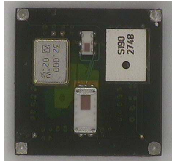
Encapsulated module with exposed chip antenna and MEMS microphone
