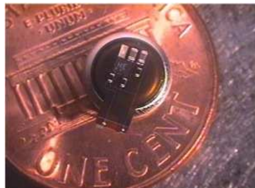
Fig. 2. LED control circuit fabricated on a polyimide substrate and mounted on a small Li battery
