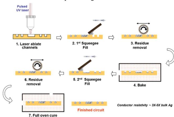
Figure 2. Fabrication steps for nanoparticle silver conductors
