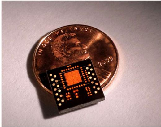
Figure 8a. 10mm x 10mm module containing microcontroller, voltage regulator and I/O switch.
