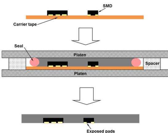
Figure 6a. Encapsulation process for SMD leadless components. Top: placement on tape carrier; Center: epoxy casting, and Bottom: removal of carrier tape.
