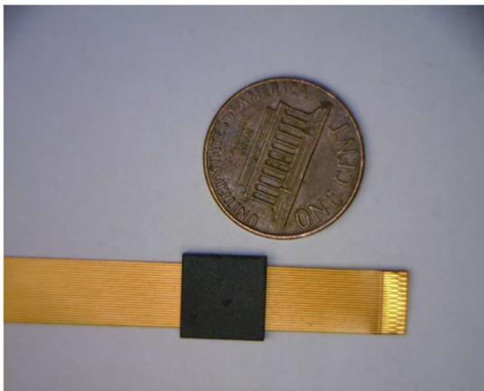
Figure 8c. Microcontroller and voltage regulator mounted on and connected to a 23-conductor flat cable.
