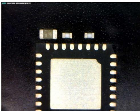
Figure 6b. Photograph of active device in QFN package with three surface-mount passive components above.
