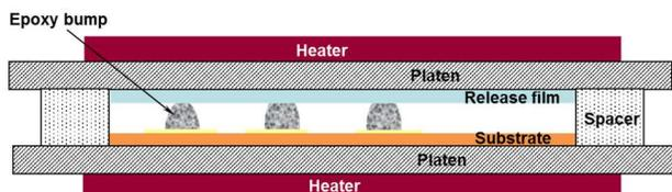
Figure 4. Bump leveling and curing fixture.
