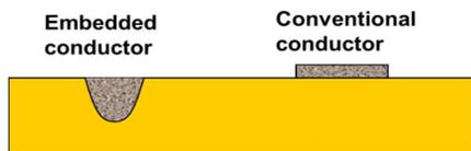
Fig. 1. Embedded conductor compared to conventional jetted or etched conductor.
