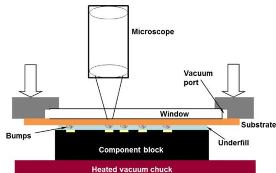
Figure 7. Sketch of bonder used for attaching interconnect substrate to component block.
