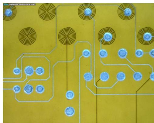
Figure 5. Bumped conductor pattern. Darker conductors are on the backside.
