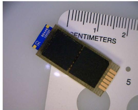
Figure 8b. Wireless sensor with two modules containing microcontroller and accelerometer. Modules are mounted on FR4 board with radio and battery on backside.
