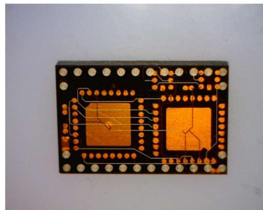
Figure 8d. 8mm x 12mm module containing microcontroller, 16-channel LED driver, and two switch IC's.
