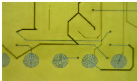
Figure 3. Two-sided conductor pattern showing vias, conductor widths of 15 and 50 micrometers, and spiral pads. The 50 micrometer conductors were fabricated with 3 parallel assemblies of 15 micrometer conductors. Darker traces are on the back side.
