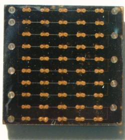
Figure 9. Fifty-element daisy chain constructed from 0201 zero-ohm resistors used for thermal cycling tests.
